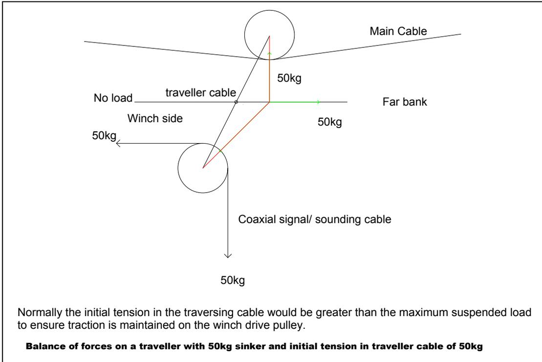
pulley, a torque is applied to this pulley in proportion to the tension in the traversing cable caused by the load on the sounding cable. A load limiter may be incorporated in this pulley to allow it to slip at a preset tension in the sounding cable. The figure above shows the action of the forces at the traveller. If it is not practicable to add a load limiter to the winch, it is possible to incorporate it into the traveller.
